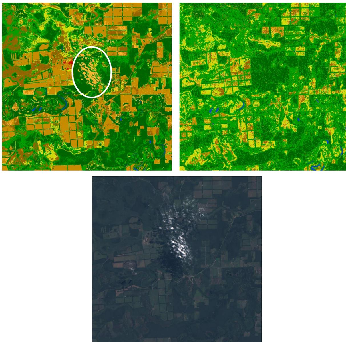
Figure 42 Details of the classification maps obtained from the classification of optical (top left) and SAR data (top right), indicating the impact of a residual cloud on the former. A true-color composite of the optical image is also shown (bottom).
