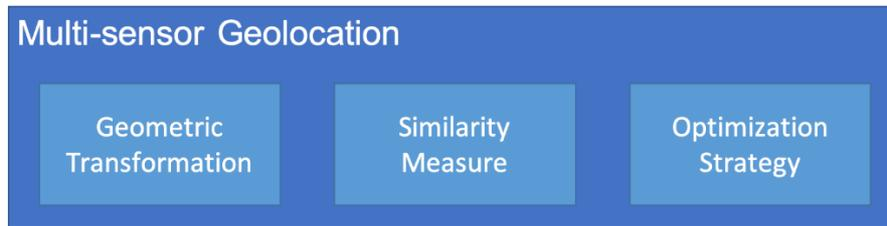
Figure 63. Composition of the multisensor geolocation process.
