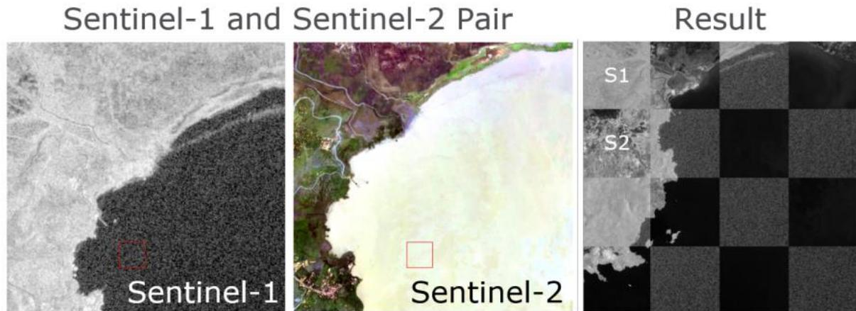
Figure 92. Details of the spatial feature in one of the tiles in which the granule 37PCP is divided into. On the left, Sar image; in the centre, optical image; on the right, a checkerboard representation of the results achieved by the registration, even with very few features available.
